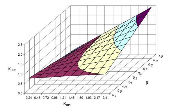
Fig. 4 – Values of dimensionless criterion of energy efficiency of large capacity HPP with electric drive for the cases of variable load of HPI, on condition of electric energy consumption from energy system of Ukraine
