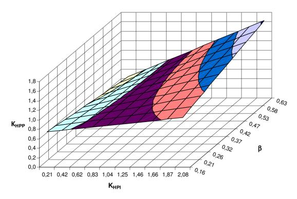
Fig. 12 – Values of dimensionless criterion of energy efficiency of large capacity HPP with electric drive for optimal values of HPI load share, on condition of electric energy consumption from GTI
