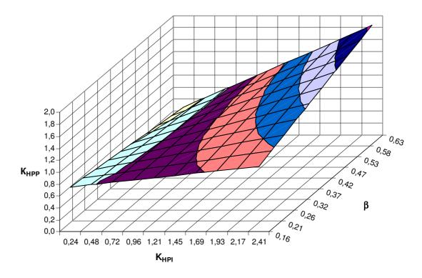
Fig. 10 – Values of dimensionless criterion of energy efficiency of large capacity HPP with electric drive for optimal values of HPI load share, on condition of electric energy consumption from energy system of Ukraine
