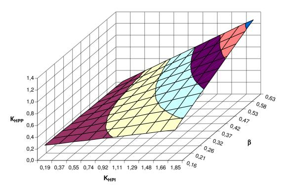
Fig. 9 – Values of dimensionless criterion of energy efficiency of small capacity HPP with electric drive for optimal values of HPI load share, on condition of electric energy consumption from GTI
