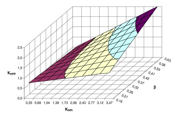
Fig. 11 – Values of dimensionless criterion of energy efficiency of large capacity HPP with electric drive for optimal values of HPI load share, on condition of electric energy consumption from SGI
