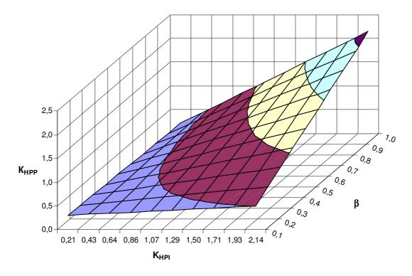
Fig. 1 – Values of dimensionless criterion of energy efficiency of small capacity HPP with electric drive for the cases of HPI variable load, on condition of electric energy consumption from energy system of Ukraine
