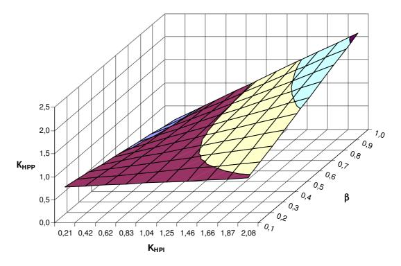
Fig. 6 – Values of dimensionless criterion of energy efficiency of large capacity HPP with electric drive for the cases of variable load of HPI, on condition of electric energy consumption from GTI
