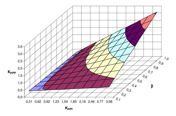
Fig. 2 – Values of dimensionless criterion of energy efficiency of small capacity HPP with electric drive for the cases of HPI variable load, on condition of electric energy consumption from SGI
