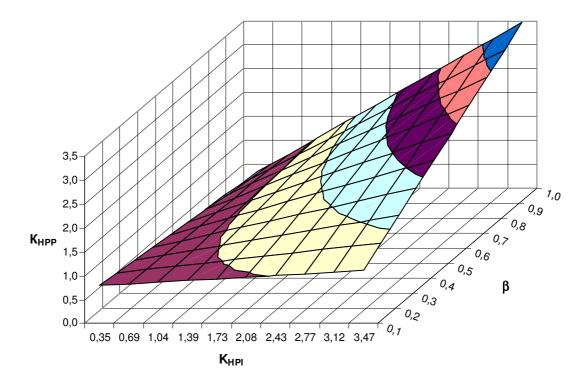
Fig. 5 – Values of dimensionless criterion of energy efficiency of large capacity HPP with electric drive for the cases of variable load of HPI, on condition of electric energy consumption from SGI
