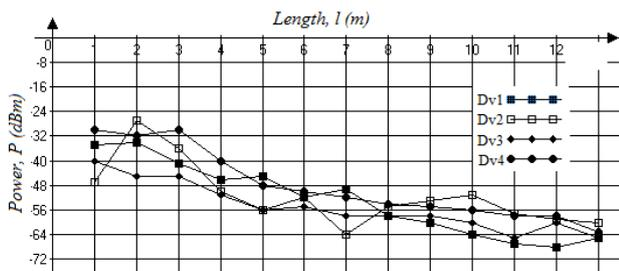
Figure 3. Dependence of signal strength on distance
