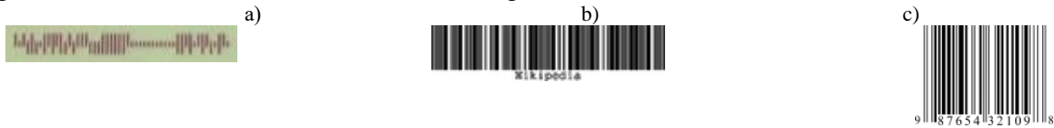
Fig. 1. Examples of the linear bar codes: a) Australia Post bar-code; b) Codabar; c) Code 25 – Interleaved 2 of 5
