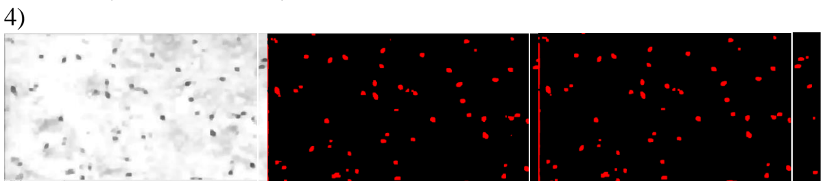
d) Gray Morphology_1: Modifies the shape of objects in an image. (Operation: Erode – Structuring Element cross 3×3, Iterations - 4) e) Gray Morphology 2: Modifies the shape of object in an image. (Operation: Dilate – Structuring Element square 3×3, Iterations - 3) f) Gray Morphology_3: Modifies the shape of object in an images. (Operation: Close – Structuring Element square 9×9)
