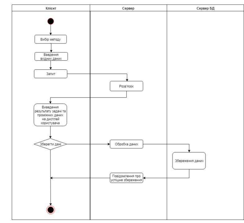
UML-diagram of the distribution of functionality when placing the solution algorithm on the client side
