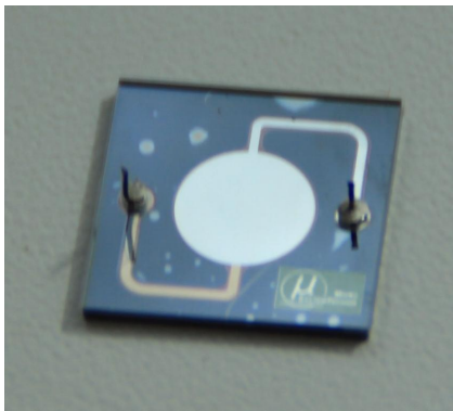
Figure 1. Schematic diagram of the frequency transducer pressure with sensitive MEMS capacitor.
