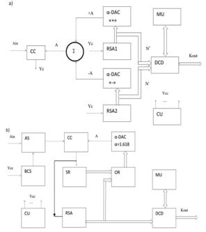
Fig.1. Structural diagrams of bitwise self-calibrated ADC of accelerated speed with weight redundancy on the base of: a) CSWR (1, 1); b) CSWR (0, 1)
