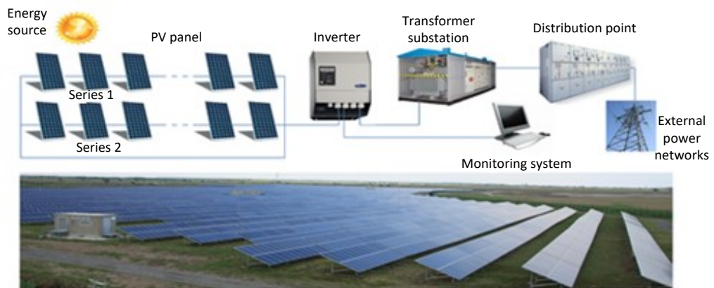
Fig. 2.3 Technological scheme of PV
