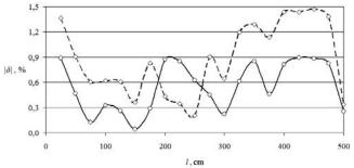
Fig.4. Dependence of absolute values of the relative error  $|\delta|$  from the measured distance I: with consideration of environmental parameters —o and without consideration of environmental parameters --- $\diamond$
