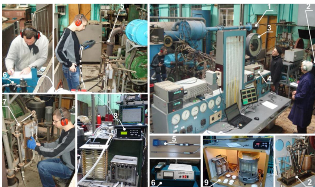
Figure 1. General view of the test bench of the automobile diesel 4ChN12/14 with universal system of ecological diagnostics:
