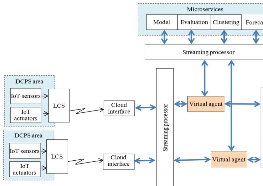
Figure 3. Architecture of coordination system using microservices
