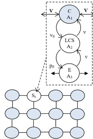
Figure 1. DCPS hypergraph with decentralized coordination of local control systems
