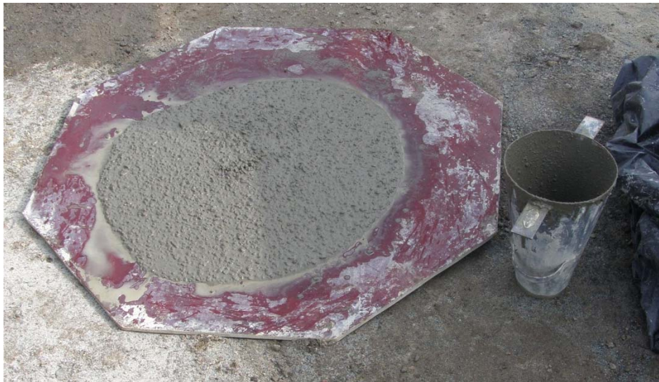
Figure 3 – Self-compacting concrete (SCC) based on Sika ViscoCrete-20 HE superplasticizer. Cone slump test of concrete
