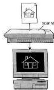
A colour scanner operates by using three rotating lamps, each of which has a different coloured filter: red, green and blue. The resulting three separate images are combined into one by appropriate software.
