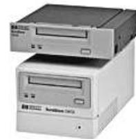
DAT (Digital Audio Tape) devices are commonly used for backups. The DAT tapes that they use can backup enormous amounts of data (i.e. over 4 GBytes per tape). The devices are also fast and reliable.
