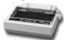
printing graphics. As a result, the dot matrix printer has now largely been replaced by the inkjet printer. Dot matrix printers are used for high volume / low quality printing, e.g. printing company pay slips.
