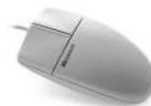
be a competent mouse user. There are many different types of mice, a commonly used model now has a small wheel on it which when combined with the correct software allows additional functionality and fine control over the use of your applications.
