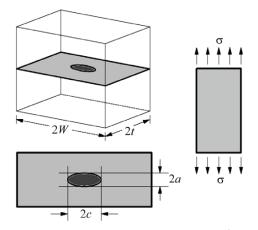
Fig. 6. Loaded slab with internal elliptical central crack: 2W - length of the slab; 2t - its width; 2a - length of the crack; 2c - its width;  $\sigma$  - applied force
