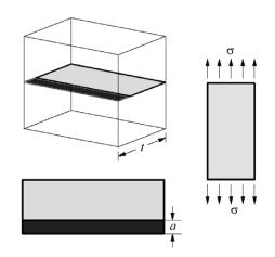
Fig. 2. Loaded slab with external edge crack: t- width of the slab; a- length of the crack;  $\sigma-$  applied force
