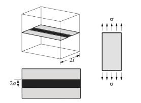
Fig. 1. Loaded slab with a central longitudinal crack: 2t - the width of slab;  $2a - the length of slab; \sigma - applied force$
