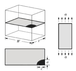
Fig. 5. Loaded slab with quarter-elliptical angular crack: W - length of the slab; t - its width; a - length of the crack; c - its width;  $\sigma$  - applied forces
