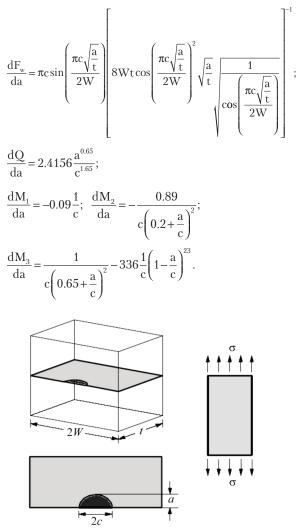
Fig. 4. Loaded slab with half-elliptical edge crack: 2W – length of the plate; t – its width; a – length of crack; 2c – its width;  $\sigma$  – applied force
