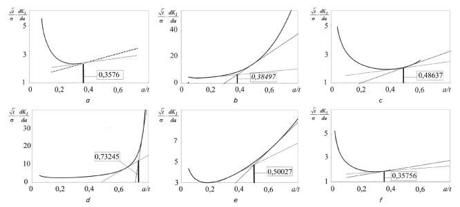
Fig. 7. Determining characteristic values (a/t)\* for the cases of propagation of crack-like defects at the tension of slab: a – with a central longitudinal crack; b – with external edge crack; c – with two external edge cracks; d – with a half-elliptical edge crack; e – with a quarter-elliptical angular crack; f – with an internal elliptical central crack
