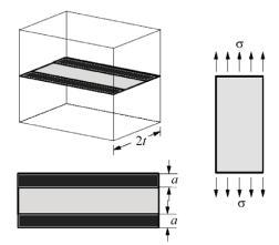
Fig. 3. Loaded slab with two external edge cracks: 2t - width of the slab; a - length of crack;  $\sigma$  - applied force
