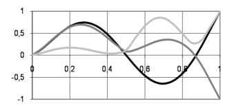
Figure 2: – Forms of free oscillations boom with rigid connections sections.
