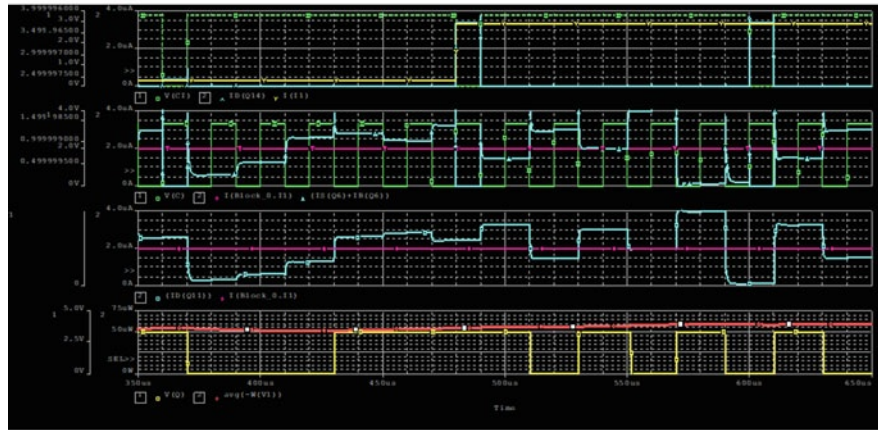
Fig. 4.21 (a) Simulation result for two input currents 100 nA and 150 nA, corresponding output Gray codes {000001} and {000011}; the blue line in the third trace is output current of the block for six-digit ADC, the violet line is the threshold current; the yellow line in the fourth trace is the output voltage of the block that corresponds to output code (a time interval for the first code 370–490 \mu s (six digits by 20 \mu s), a time interval for the second code 490–610 \mu s); the red line is the power consumption of about 40 \mu W. (b) Simulation result for two input currents and corresponding output Gray codes {000111} and {010101}; the consumption power is about 40 \mu W
