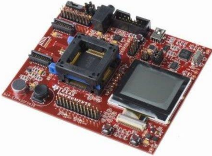
Fig. 3. Microcontroller unit on board MSP-EXP430F5438
