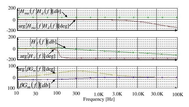
Fig. 7. Simulation results: frequency response of MagAmp post-regulator control loop components. Top trace: MagAmp frequency response including the delay,  $H_{ma}(f)H_d(f)$ ; middle trace: output filter frequency response,  $H_f(f)$ ; bottom trace: control circuit frequency response  $\beta G_m(f)$ .
