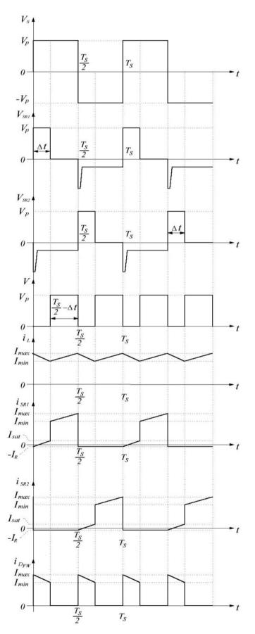
Fig. 3. Waveforms of a push-pull MagAmp regulator
