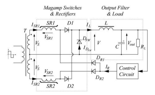
Fig. 2. Push-pull MagAmp regulator circuit
