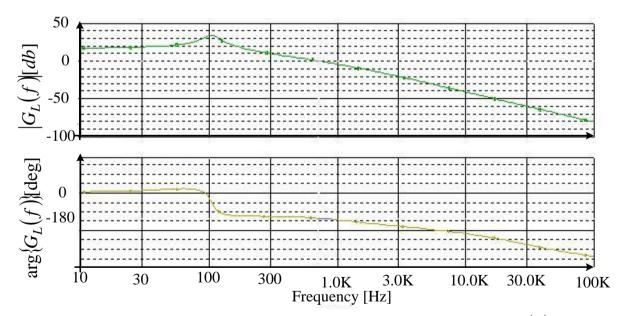
Fig 8. Simulation results: overall frequency response of MagAmp post-regulator loop-gain  $G_L(f)$ . Top trace: Magnitude [db]; bottom trace: Phase [deg]
