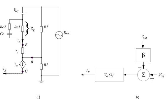
Fig. 6. MagAmp controller equivalent circuit a) and its small signal model b)
