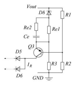
Fig. 4. Control circuit of MagAmp post-regulator
