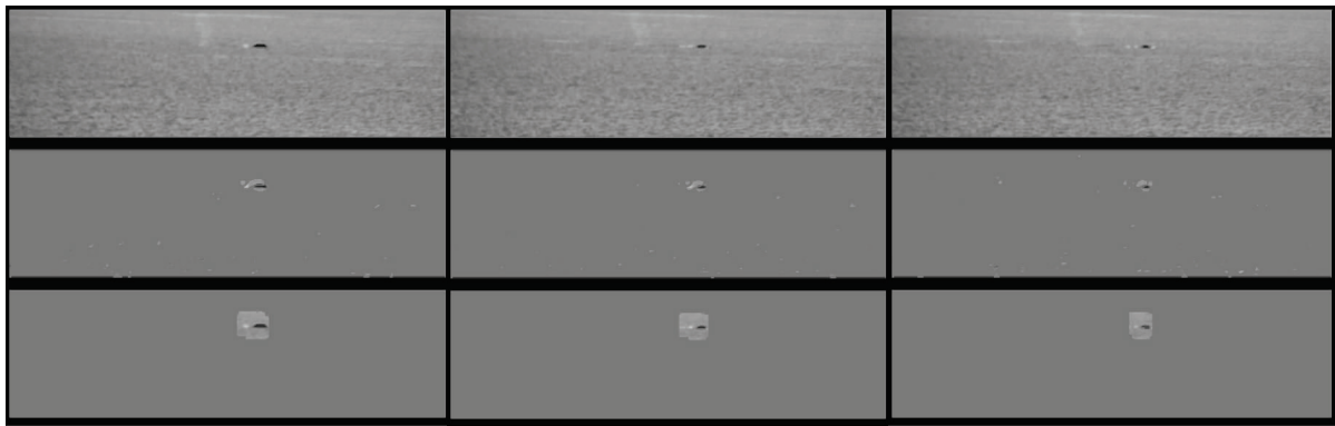
initial images; middle positions – images filtered by IRF; low positions – images filtered by correlative filter
