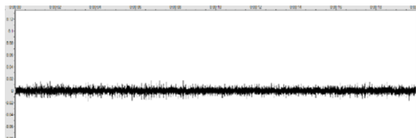
Fig. 7. Oscillogram of vibration acceleration of the controlled axle of the MTZ-80 tractor at installation of the accelerometer on a sliding pipe of the axle
