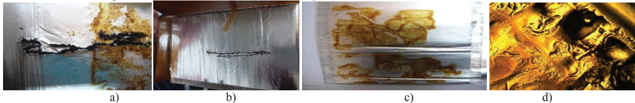
FIGURE 3. Traces of the breakdown of the section with deformation of the foil and dielectric film and traces of decomposition of the dielectric film and liquid dielectric (a); traces of electrical breakdown of the section, which begin at places of deformation of the organic film and reach the surface of the section (b);Traces of decomposition of organic film and liquid dielectric without visible breakdown (c); and Traces of the beginning of the breakdown of a dielectric film, with traces of its decomposition in a liquid dielectric, at the point of its deformation, detected under a microscope (d).
