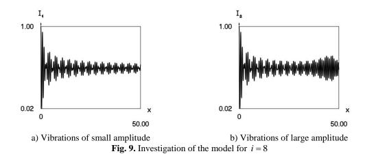
Graphical relationships show the importance of use of more precise equation for estimation of intensity of time averaged reflection moiré images when vibrations are of large amplitude.
