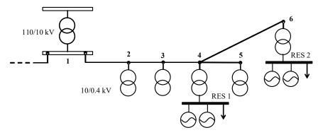
Fig. 6. Diagram of the electrical network 10 kV
