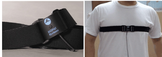
Fig. 6 Respiratory effort transducer SS5LB and its location
