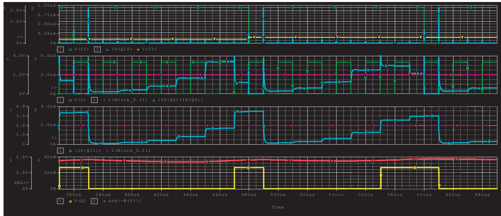
Fig. 3. a) Simulation result for two input currents 100\text{nA} and 150\text{nA} , corresponding output Gray codes \{000001\} and \{000011\} ; the blue line in the third trace is output current of the block for six digits ADC, the violet line is the threshold current; the yellow line in the fourth trace is output voltage of the block that corresponds to output code (a time interval for the first code 370\mu\text{s} - 490\mu\text{s} (six digits by 20\mu\text{s} ), a time interval for the second code 490\mu\text{s} - 610\mu\text{s} ); the red line is the consumption power about 40\mu\text{W}
