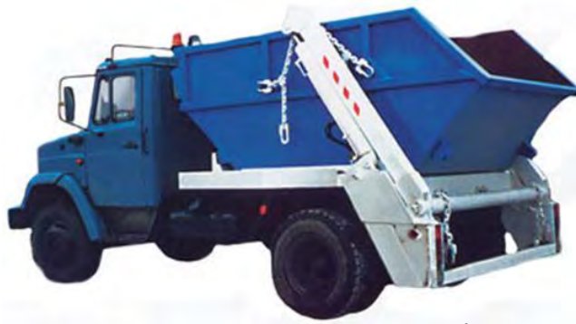
Fig. 3. Container garbage truck for containers with a volume of 7.6 m 3 for collecting large-sized waste
