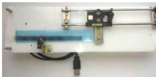
Fig. 2. General view of the current model of the linear displacement sensor on the moire effect
