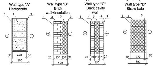
Fig 1. Considered wall types compositions «A»-«D» (1 – internal lime-sand plaster, 2 – hemcrete, 3 – external lime-sand plaster, 4 – honeycomb brick, 5 – mineral wool, 6 – strawbale panel, 7 – autoclaved aerated concrete (AAC), 8 – plywood, 9 – ecofiber)
