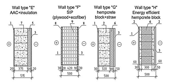
Fig 2. Considered wall types compositions «E»-«H» (1 – internal lime-sand plaster, 2 – hemcrete, 3 – external lime-sand plaster, 4 – honeycomb brick, 5 – mineral wool, 6 – strawbale panel, 7 – autoclaved aerated concrete (AAC), 8 – plywood, 9 – ecofiber)
