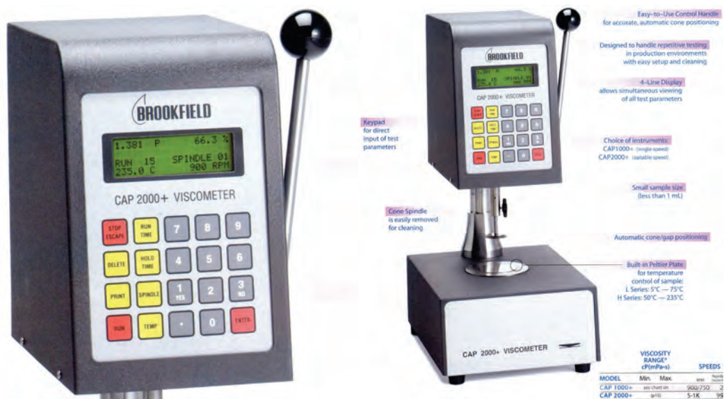
Fig. 13. The applied Brookfield viscometer CAP2000+ and some its characteristics [22]
