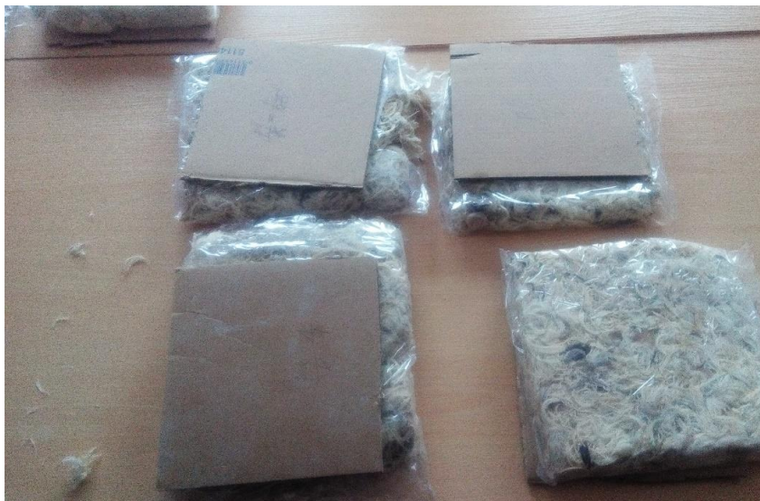
Figure 5. Composites made of hens' feathers and hydraulic lime
