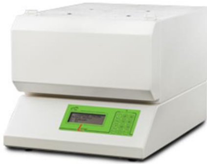
Figure 2. The computerized thermal conductivity measurement device - heat flow meter LaserComp FOX 200
