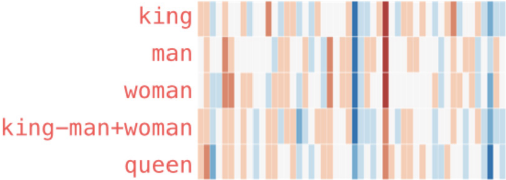
Figure 5.24 – Result of operations with embeddings "king" – "man" + "woman" and comparison of the result with embedding of the word "queen" (from the blog )
