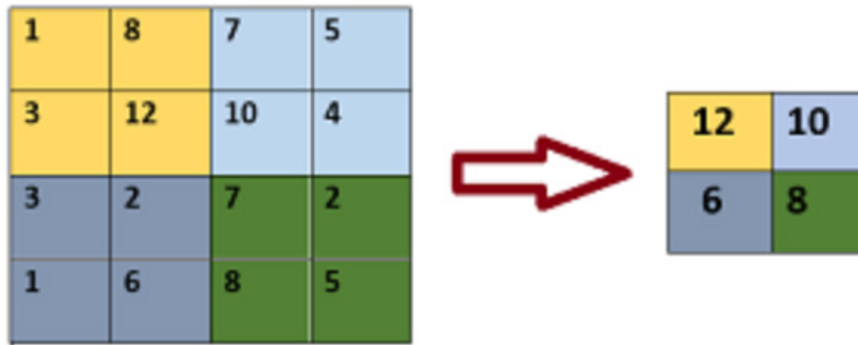
Figure 5.10 – Example of MaxPooling2D(pool_size=(2, 2), strides=None, padding="valid") [41]
