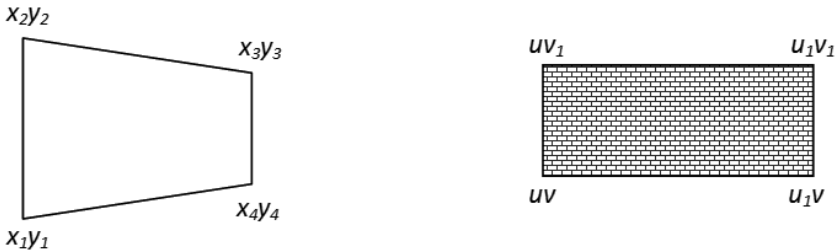
Fig. 4.20. A polygon with opposite sides parallel to the Y axis and a sample texture
