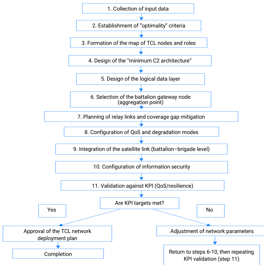
Figure 2. Generalised scheme of the algorithm for designing and configuring a TCL communication network under EW conditions
