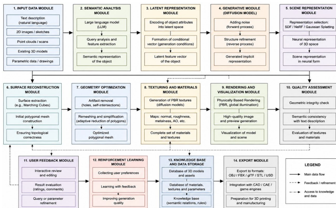
Drawing 1 - Modular architecture of a system for generative synthesis of three-dimensional objects
