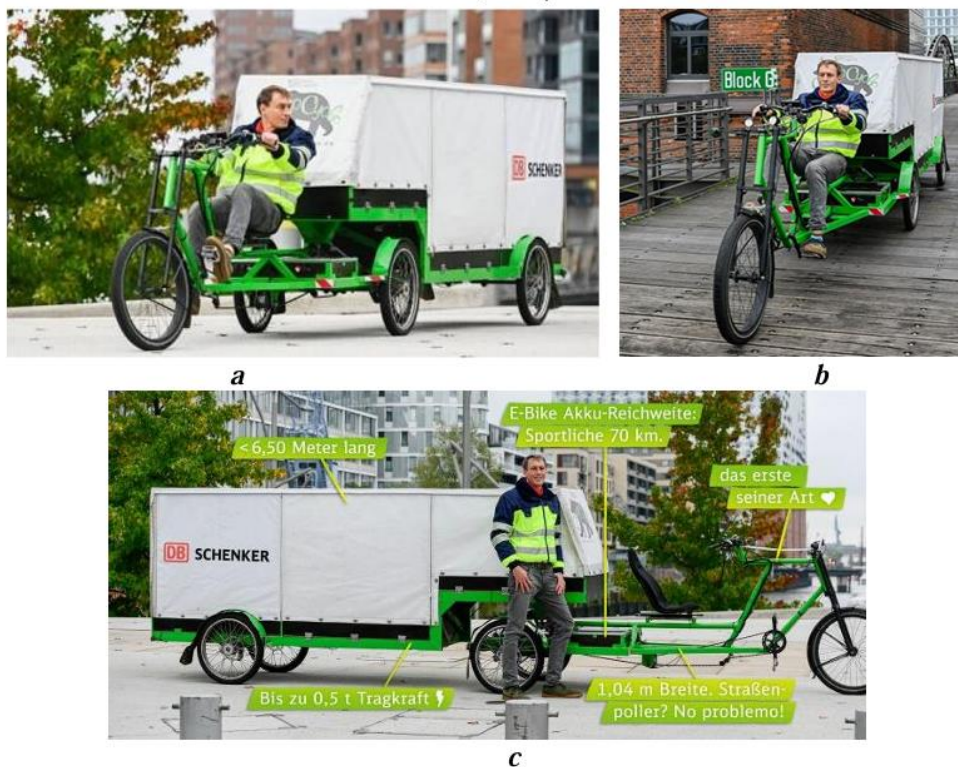
Fig. 1. DB Schenker's Velogista cargo bike, which is equipped with an electric drive and can transport up to 250 kilograms of cargo with a loading volume of up to 1.6 m 2 [5]: a – side view of the bike moving around the city; b – front view of the bike moving around the city; c – general view of the bike, with a length of 6.5 meters and a load capacity of up to half a ton, the Cargo Bike is a real "megalin" among cargo bikes
