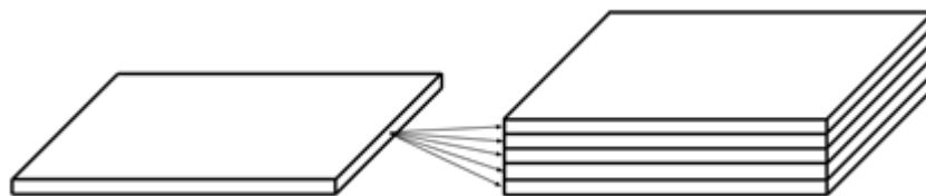
Figure 6. Illustration of voxel model formation based on binary slice images
