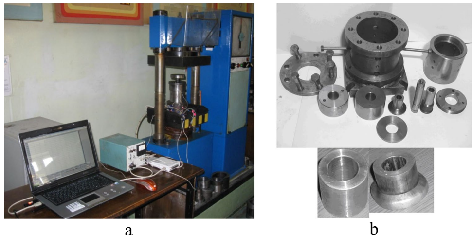
Fig. 4 Experimental stand based on the test press MS-500 (a). Technological equipment and specimens for deforming (b)
