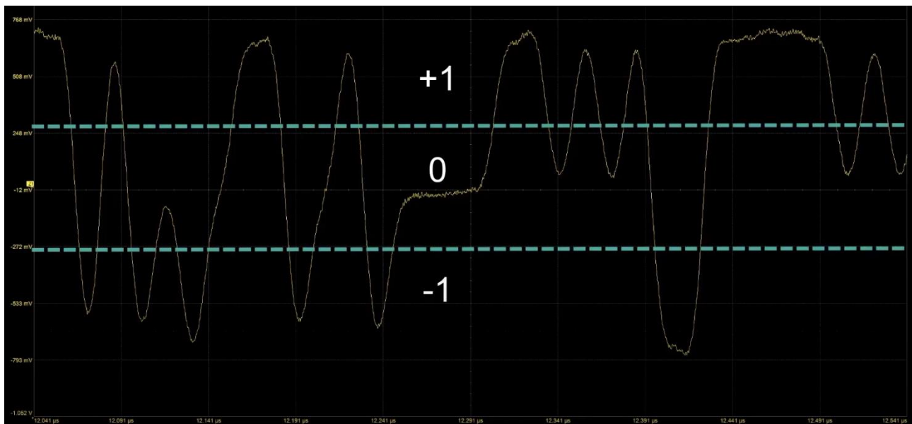
Figure 2 Example of signal conversion in PAM3
