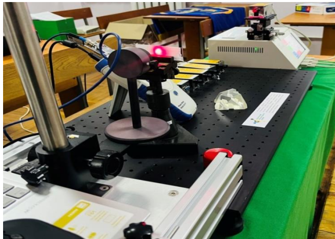
Figure 2. Laser stand for determining the absorption coefficient of biotissue in IR (830 nm) and red (658 nm)
