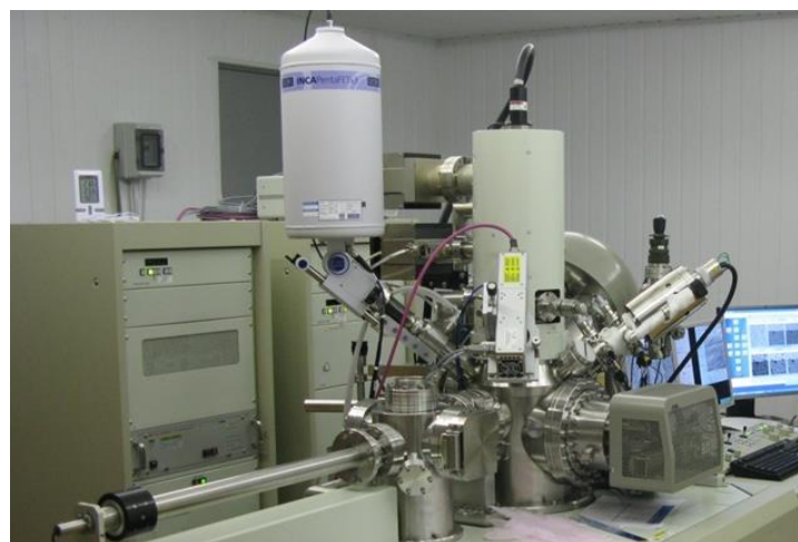
Figure 2. Auger-microprobe JAMP-9500F (JEOL, Japan): high-resolution field emission electron gun scanning electron microscope (1); Auger electron spectrometer with high resolution (2); Ar-ion gun (3); energy dispersive X-ray spectrometer INCA PentaFETx3 (4); microfocus X-ray tube with capillary (5).
